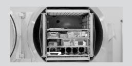
**HeVACool** systems are mainly used in the aerospace industry and simulate controlled the environmental parameters pressure and temperature of space. Materials, components and assemblies can be qualified and tested for their suitability.
